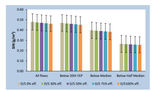
Figure 1: Predicted average SIN concentrations downstream of the EWWTP, assuming 0%, 30%, 50%, 75% and 100% removal of nitrate-nitrogen from the effluent.
